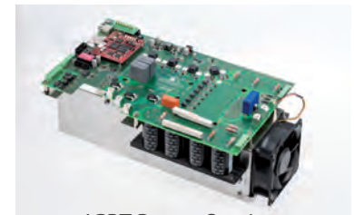
IGBT Power Section
